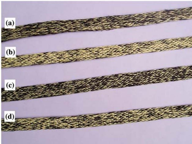
Fig. 1 Photos of 3-D braided hybrid fabrics with different carbon to Kevlar ratios (a) 3:2 (b) 1:2 (c) 3:1 (d) 3:4
